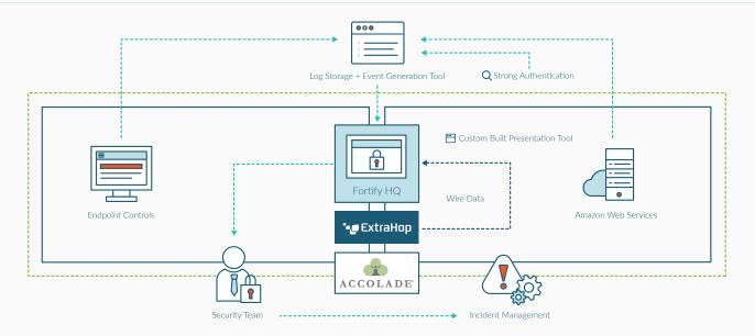
By triggering a precise packet capture for suspicious events, and then sending that data to an open- source IDS solution using the ExtraHop Open Data Stream (ODS), Sheward and his team now have real-time intrusion alerting -- and the digital evidence needed to investigate incidents -- without requiring extensive customization.
