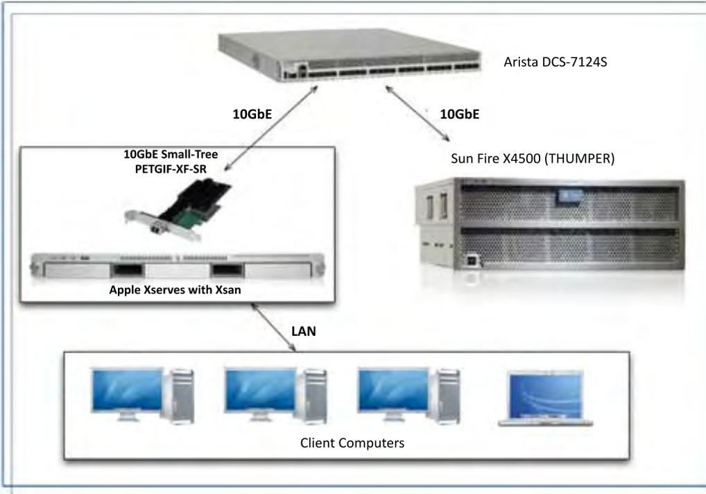
Given the limitations of Fibre Channel and 1 Gigabit based iSCSI storage systems, the BBC selected the Sun X4500 x64 based server (code name Thumper), which offers 2GB disk I/O per second using 48x 1TB disks at a cost of less than 1€ per Gb for the complete server.
